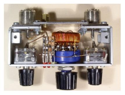
The ATU circuitry is placed in precise shielded enclosure. The body is made from aluminium milled along bending lines. Top and bottom covers are separate parts fixed with M3 screws to the body. All electronic parts fit perfectly inside. The coil is soldered directly to the rotary switch pins. SWR detector is mounted on the small piece of universal board. The current transformer uses very small FT23-43 core. I would probably use the bigger one for easier winding!
