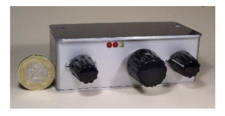
Hans designed his ATU for field day in 2003. It is really tiny; 86x33x70mm. Despite small dimensions provides wide matching range and is equipped with unique LED SWR indicator.
